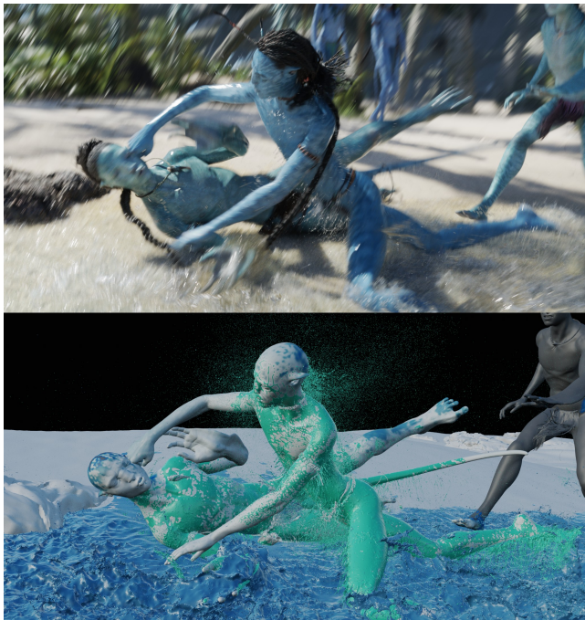
Figure 8: We employed the thin film approach of [Stomakhin et al. 2019] to run high resolution FLIP simulations (voxel size \leq 1 mm) on characters’ surfaces to achieve believable dripping effects. The bulk water surface (blue) was used to source and sink thin film particles (green) for efficiency, limiting the simulation to areas of visual significance. ©Disney and Wētā FX.
